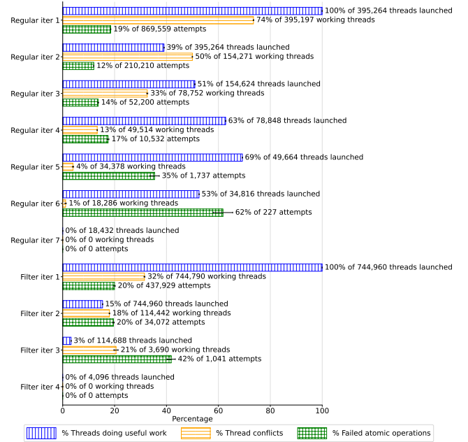
Figure 2: Bar plot of metrics derived from ECL-MST profiling data for the amazon0601 input. Error bars show 95% confidence intervals around the median.
