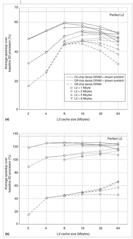
Figure 4. Performance with varying L2 and L3 cache sizes: integer (a) and floating-point (b). The straight dashed line near the top illustrates the performance of the ideal case of a perfect L2 cache, in which all accesses hit in the L2.
