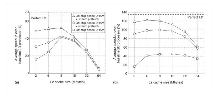
Figure 3. Average performance with varying L2 cache sizes: integer (a) and floating-point (b). The straight dashed line near the top illustrates the ideal case of a perfect L2 cache, in which all accesses hit in the L2.
