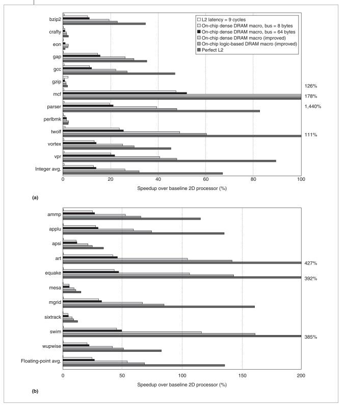
Figure 2. Benchmark performance of 3D processors with a hypothetical 2-cycle reduction in L2 hit latency: integer (a) and floating-point (b). The figure shows four possible scenarios of stacked on-chip main memory with different memory bus widths and compares both dense DRAM and logic-based DRAM macros. "Improved" indicates a memory controller latency improvement of 50%. We also plot the perfect L2 case, in which all accesses hit in the L2.
