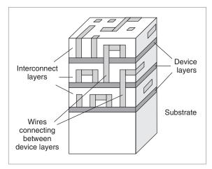
Figure 1. 3D ICs consist of planar device layers separated by silicon dioxide or other insulating materials and interconnected by short, vertical wires.
