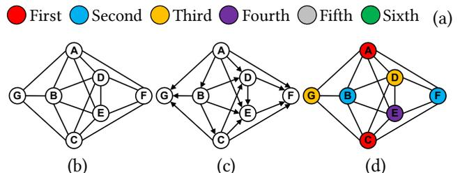
**Figure 1:** Assumed color order (a), sample graph (b), LDF-imposed DAG (c), and greedy coloring (d)
