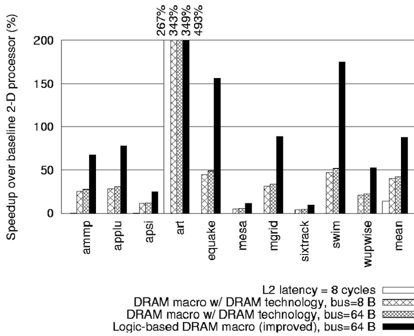
Fig. 2. Integer (top) and floating-point (bottom) benchmark performance of 3-D processors with (1) hypothetical 2-cycle reduction in L2 hit latency, and (2) three possible scenarios of on-chip, stacked main memory with different memory bus widths. The last case represents logic-based DRAM (less dense but much faster than standard DRAM) with improved memory controller capabilities.
