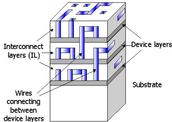
Fig. 1. Three-dimensional integrated circuits (3-D ICs) consist of planar device layers separated by silicon dioxide (or other insulating materials) and interconnected by short vertical wires.
