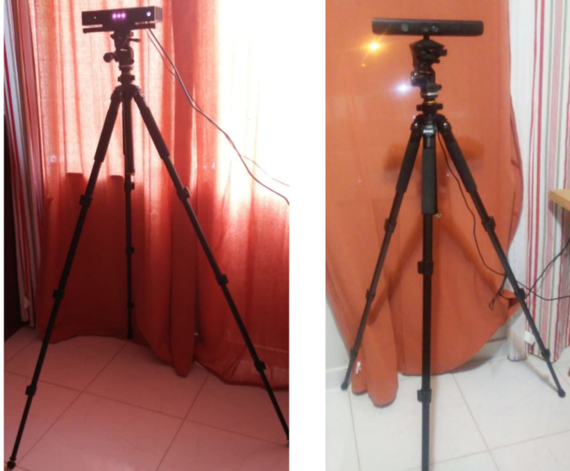
Figure 2.13: Kinect 2 (left) and Kinect 1 (right) assembled on a tripod, in the configuration used for capture experiments.
