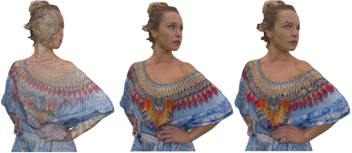
Figure 3.1: Voxelization effects, from left to right, with a too small voxel size, with a proper voxel size, and with an oversized voxel.
