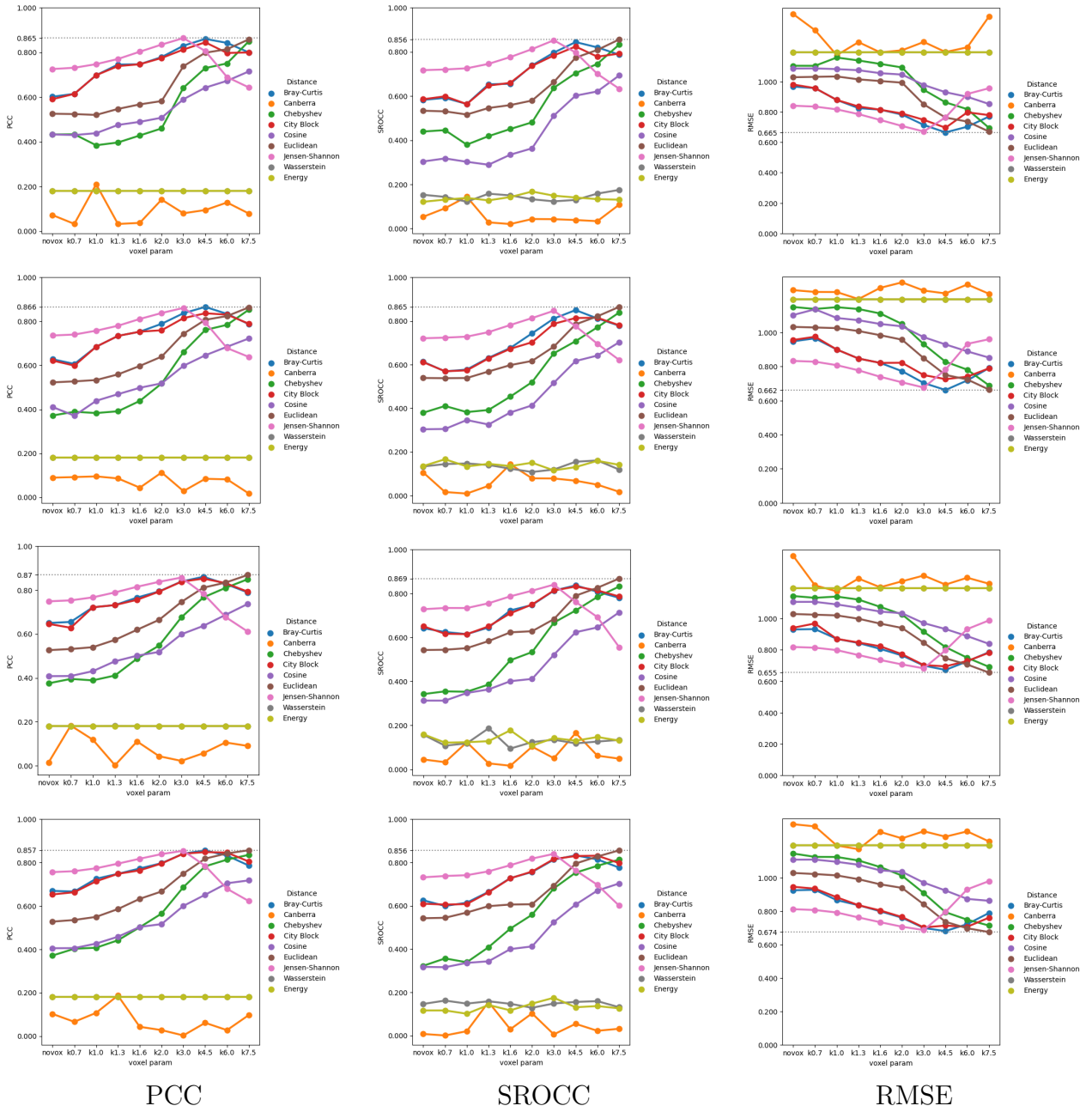
Figure 4.18: D3 LLP 16 bits descriptor performance with different histogram distances evaluated, with each row representing the LLP with 6, 8, 10 and 12 neighbors, respectively.
