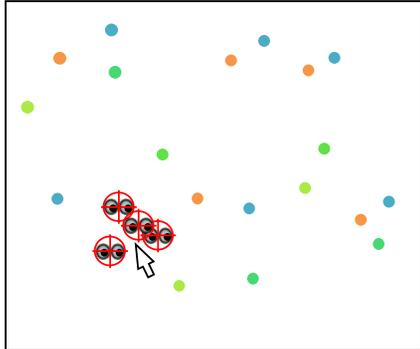
**Figure 9.** Nearest local calibration point changes with jittery eye gaze center coordinates. An offset vector is associated with each point.
