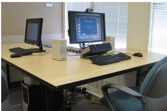
Figure 2. The prototype ATM authentication interface running on a computer in our usability lab. The eye tracker is positioned beneath the display.
