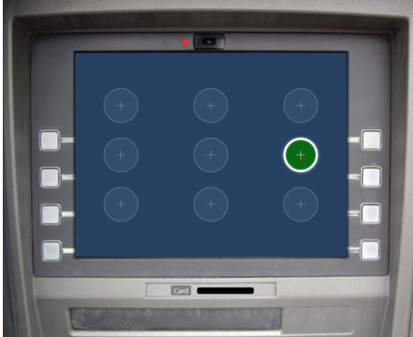
Figure 1. The user activates each circle using their gaze, while the eye tracker records eye movement data for authentication.
