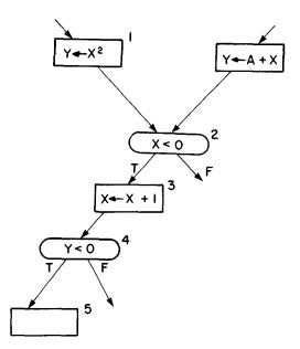
FIGURE 1. The path in this segment of a flow diagram represented by visiting the boxes in the sequence 1, 2, 3, 4, 5 is not executable. Note that  $Y \ge 0$  upon leaving box 1 and this condition is true upon entry to box 4, thus the exit labeled T could not be taken.
