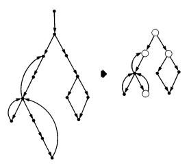
FIGURE 6. Illustration of a transformation which replaces paths consisting of a single entry and a single exit by a node. In the transformed graph open circles have been used to identify nodes representing paths in the original graph.
