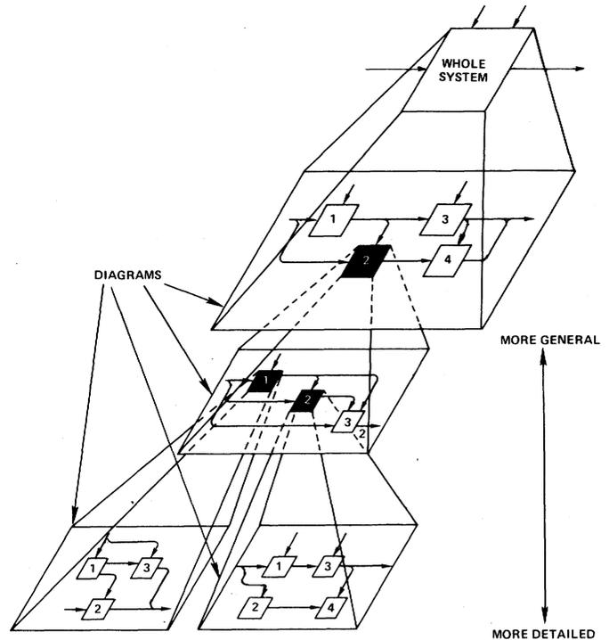
Fig. 1. Structured decomposition.
