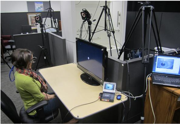
**Fig. 4** Photo taken during the data collection process. The photo shows a participant wearing the eye video recording device, as well as the rest of the experimental setup including the display unit, the data collection hardware and some of the Vicon system cameras.
