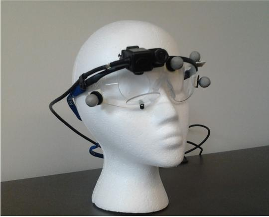
**Fig. 1** Picture of Mobile Eye-XG, head mounted, infrared monocular camera. Reflective markers used for head tracking have been attached to the glasses.
