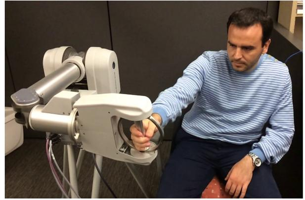
Fig. 2. A user performing a physical therapy exercise with the help of the Barrett Arm. The user is holding onto the active gimbals attached to the free end of the robotic arm.
