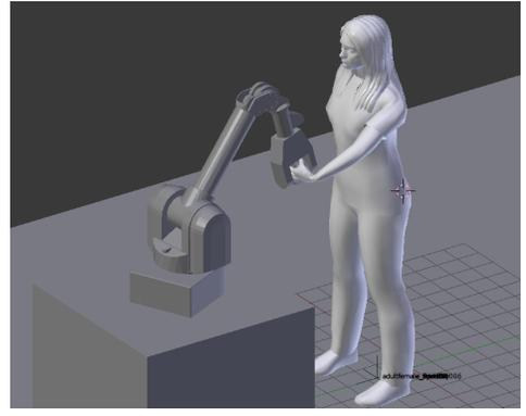
Fig. 4. Simulated 3D rendering of the robotic arm and an animated human avatar. The 3D simulation clip is used to demonstrate the correct way of exercise execution to the patients.
