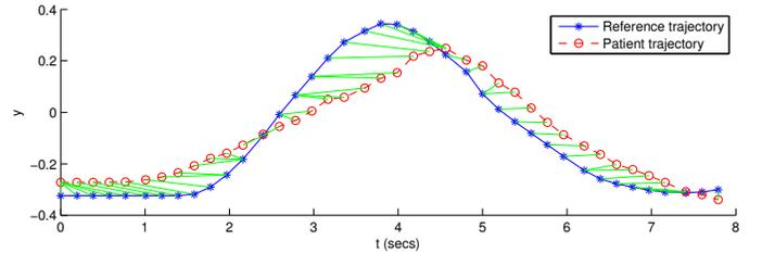
Fig. 7. Temporal trajectory alignment on axis  $y$  using the DTW algorithm.
