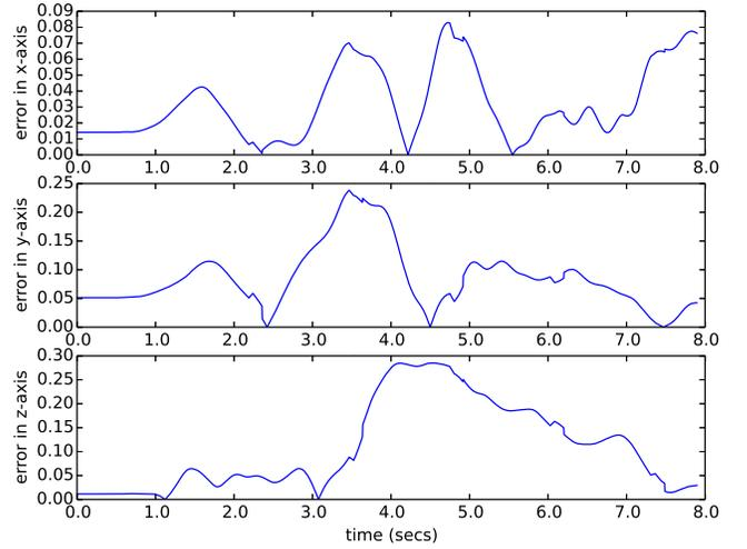
Fig. 6. Quantification of the deviation of the patient's trajectory compared to the reference trajectory, measured as error in the 3 axes of the Cartesian coordinates.
