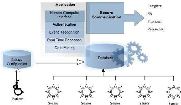
**Figure 2:** This figure shows the overview of the architecture of an assistive apartment environment. Wireless sensors collect data and share them through a database with related entities such as caregivers and physicians. They securely communicate with the environment in a real-time manner. Data mining tools are provided to analyze the collected data. Patients are allowed to configure a privacy policy on their data.
