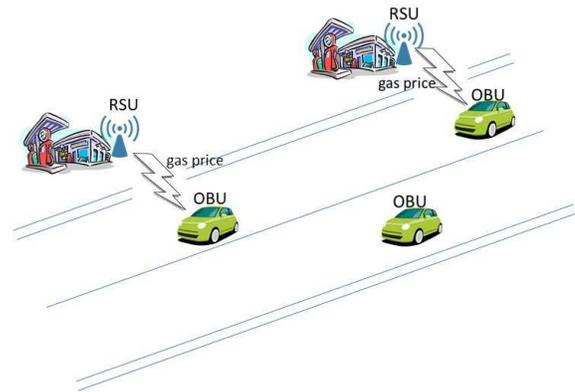
Fig. 1. RSUs at gas stations sending gas prices to OBUs in vehicles
